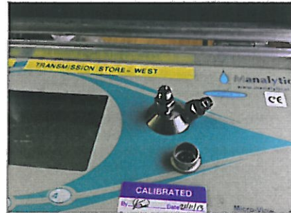
✗ No desiccant seals – sensor open to atmosphere
