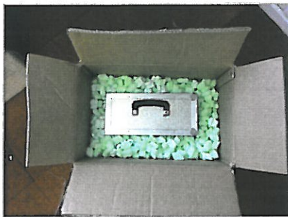
✓ Equal amount of foam chip around each side of the hygrometer
